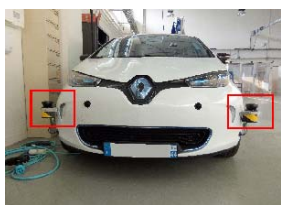
LiDARs installed on the front
