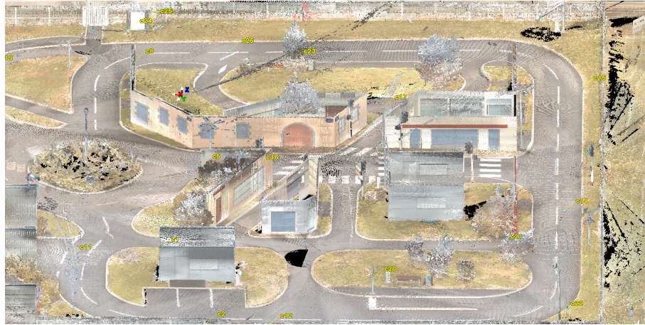
Figure 1.20: Example of scanning of the PAVIN experimentation platform obtained with the Leica P20.
