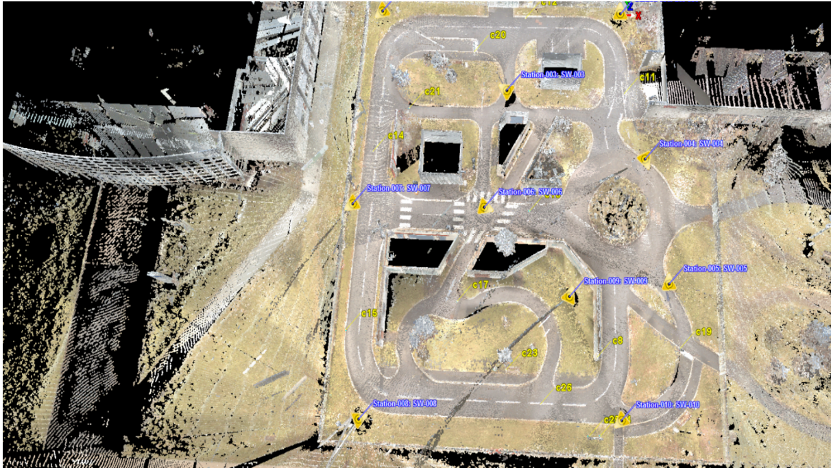
Figure 6.5: The complete PAVIN datasets comprising 10 scan stations, and over than 500 million points.
