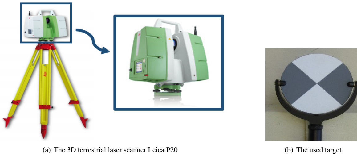
Figure 6.1: The 3D terrestrial laser scanner Leica P20 and target used for the static map building.
