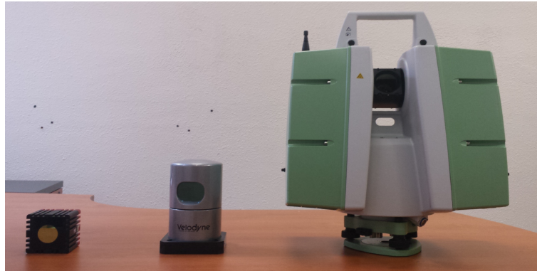
Figure 5.14: Sensors used to test the CICIP approach. From left to right: SR4000 Time-of-Flight camera, Velodyne HDL 32-E, and Leica P20 Laser.
