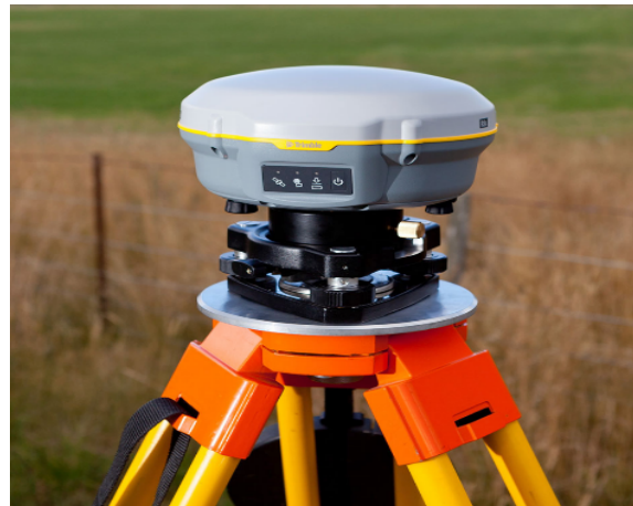
(b) GNSS Trimble: An example of a GPS terminal that allows to receive the signals emitted by the satellites, and which converts this data into geographical positions for the GPS terminal
