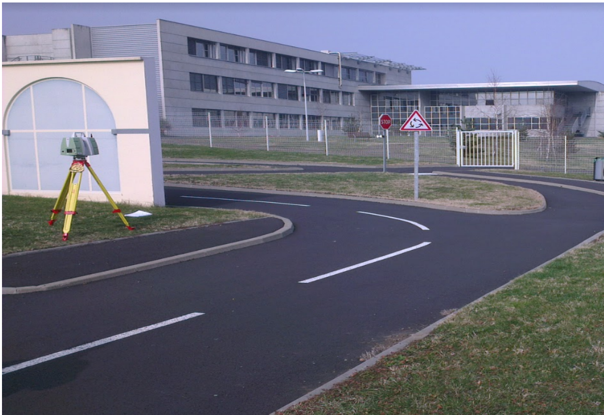
Figure 2.8: The 3D terrestrial laser scanner Leica P20 of Institut Pascal, as an example of static acquisition technique.
