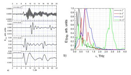
Temporal (a) and wave (b) forms of terahertz pulses generated in InAs and detected in thick GaSe sample tilted at different angles. The detection efficiency is tuned by tilting the crystal.
