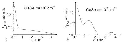
Model (a) and experimental (b) terahertz emission spectra from electron irradiated GaSe sample.
