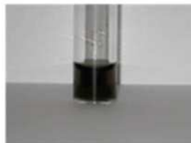
Figure 9 : dispersion aqueuse stable de nanocomposites His 6 -TagSWNT/ \text{SiO}_2 .
