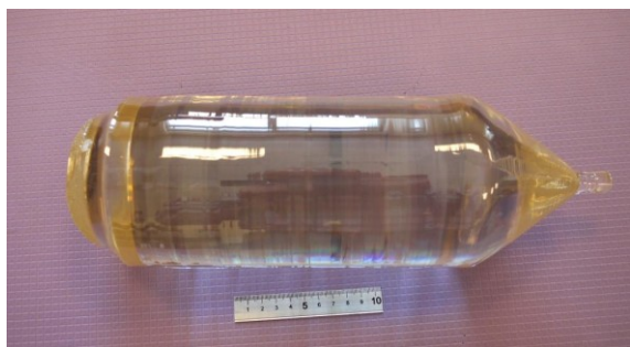
Fig. 1. CdWO_4 crystal grown by LTG Cz technique (CML ltd, Novosibirsk)
