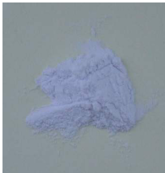
Fig. 1. The photo image of \text{Rb}_3\text{NdB}_6\text{O}_{12} powder on the grey background, as illuminated by white light.
