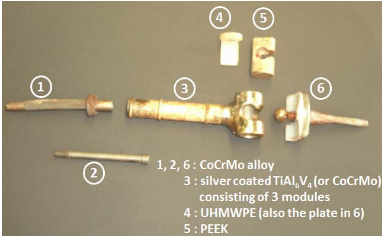
Fig. 4. Components of an explanted knee tumor endoprosthesis (after wear time of 3 years)
