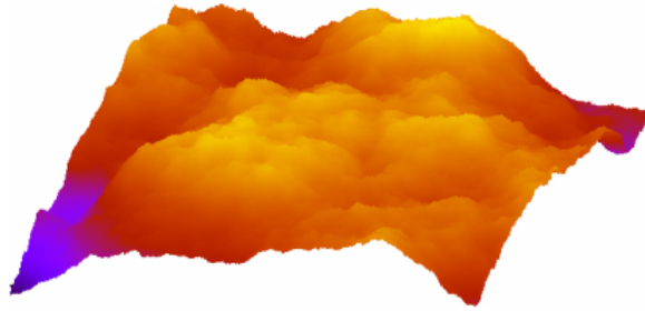
Figure 1.19: Topography picture of a surface produced by the eroding process described in Figure 1.18 after removing 76 290 layers of blocks. The surface plane consists of 2048 \times 2048 blocks. The surface is self-affine fractal with the Hurst exponent H = 1 (or fractal dimension D_f = 2 ), see Figure 1.20. The width of the removed particles (or blocks) is a = 0.1 \mu\text{m} . The surface has the rms roughness h_{rms} = 2.1 \mu\text{m} and the rms slope \kappa = 1.04 . From [40].
