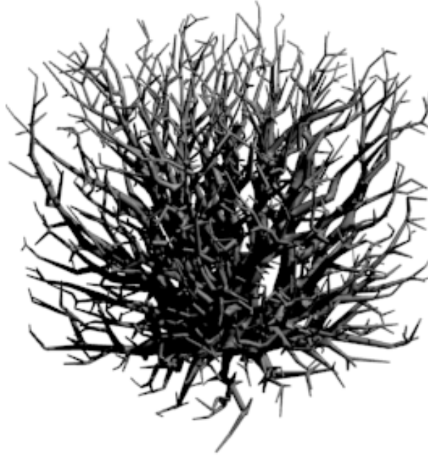
Figure 4.4: An example of a fiber structure for which the mesh generation for the fibers would be trivial, but the resulting three-dimensional elastic matrix would be much more expensive to resolve in full.
