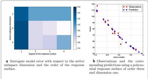
**Fig. 12** Plot **a** shows the relative error on the test dataset with respect to the active subspace dimension and the order of the response surface; plot **b** shows the observations of the test dataset and the corresponding predictions using a polynomial response surface of order three
