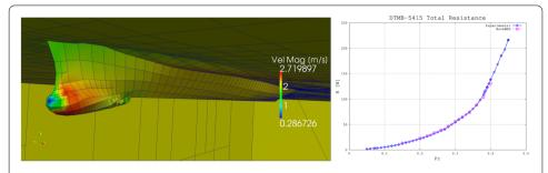
**Fig. 7** On the left, the mesh automatically generated on the surface of one of the deformed hulls obtained starting from the DTMB 5415 Navy Combatant Hull. On the right, the total resistance of the DTMB 5415 hull as a function of the Froude number associated with the surge velocity imposed in the simulations. The blue continuous line represents the experimental values presented in Olivieri et al. [33]. The values obtained in this work are represented by the dashed magenta line
