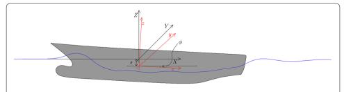
**Fig. 3** A sketch illutrating the hull-attached frame  $\widehat{xyz}$  in red and the global reference frame  $\widehat{XYZ}$  which is moving with the constant horizontal velocity of the boat. The ship here depicted is experiencing a vertical displacement s and an angular displacement characterized by the pitch angle  $\phi$
