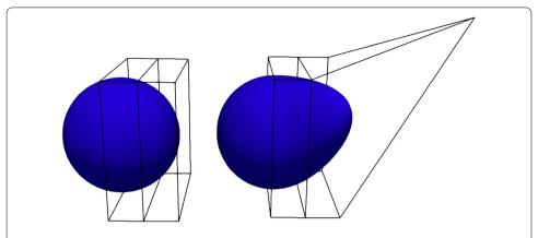
**Fig. 5** FFD morphing on a simple geometry: the sphere case. Here we move only one FFD control point in the lattice
