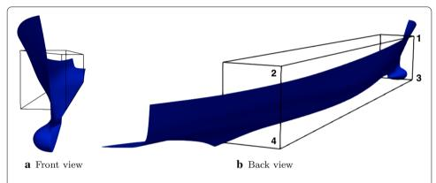
**Fig. 6** Plot **a** shows the FFD lattice over one side wall of the hull from the front, while plot **b** depicts the hull and the lattice from the back together with the numbers that identify the FFD points
