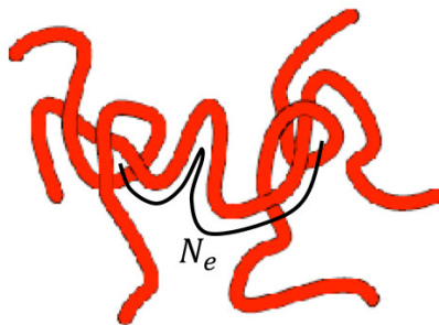
Figure 1.3: The representation of two entangled chains. The entanglement interactions slow the relative movement of center of mass of the chains and even draw them back.
