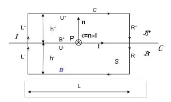
Figure 1: Burgers circuit  $C = U^+ \cup R^+ \cup R^- \cup B^- \cup L^- \cup L^+$  across an interface I separating the body  $\mathcal B$  into domains  $\mathcal B^-$ ,  $\mathcal B^+$ . 1 is the unit tangent to curve  $\mathcal C$ ,  $\mathbf n$  is the unit normal to interface I, and  $\boldsymbol \tau = \mathbf n \times \mathbf l$  the "tangent normal" to the bounded surface S and curve  $\mathcal C$ .
