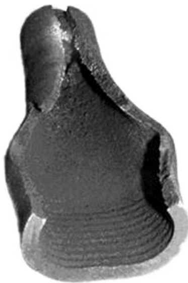
Figure 3 The view of the ampoule after explosive loading of the assembly without external tube
