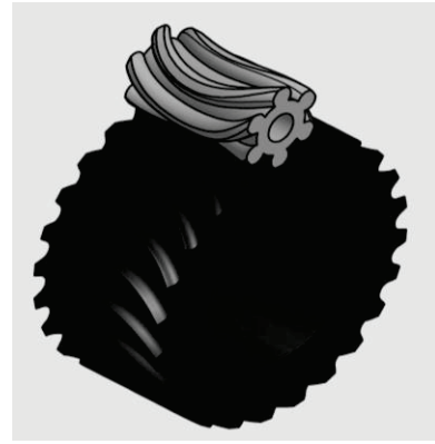
FIGURE 2. Arch teeth of the input and output parts of the gearing
