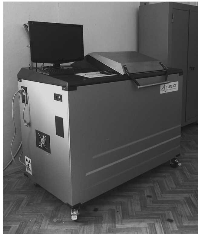
Fig. 1. The MARS scanner in the Laboratory of Nuclear Problems of the Joint Institute for Nuclear Research.
