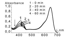
**Figure 5.** The change in the absorption spectra of the mixture  $I_2(Ph)_4$ -N-BODIPY (3×10<sup>-5</sup> M) and 1,3-DPBF (3×10<sup>-5</sup> M) upon irradiation ( $\lambda_{ex}$ =640 nm) in ethanol in oxygen atmosphere
