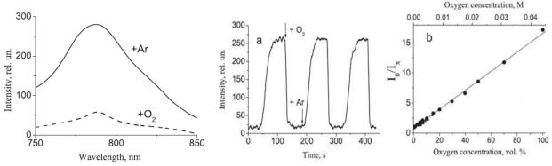
**Figure 3.** Luminescence spectra of  $I_2(CH_3)_4BODIPY$  in methyl cellulose matrix in the argon and oxygen atmospheres at  $\lambda_{ex}$ =520 nm
