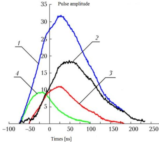
**Figure 3.** Waveforms of the laser pulses to strontium pairs: 1 – total generating momentum; 2 – impulse generation  $\lambda = 6.45 \mu\text{m}$ ; 3 – impulse generation  $\sim 3 \mu\text{m}$ ; 4 – generating momentum  $\sim 1 \mu\text{m}$ .
