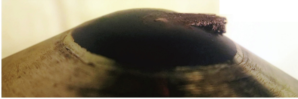
FIGURE 1. The build-up on the burnishing tool tip on the fifth run over the copper disk surface
