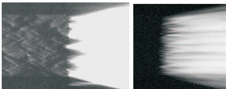
Figure 4. The streak images of the exit of the detonation wave on the free surface for the mixture of NM/M 66/34 without DETA (left) and with 2% DETA (right). Steel shell with the internal diameter of 28 mm and the length of 300 mm.
