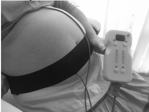
Figure 2. Layout of recorder and piezoceramic transducers adjusted to a pregnant woman's body.
