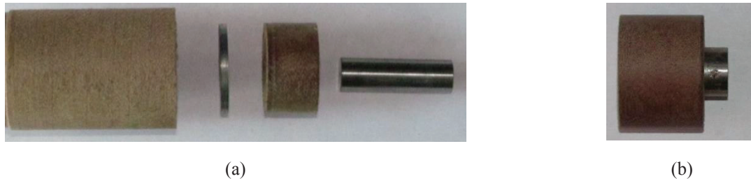
FIGURE 1. Hurlled assembly of projectile involving textolite (a) and assembly with the cermet impactor of 30 mm caliber (b) The cylindrical impactor is made from cermet material based on an alloy of tungsten-cobalt-nickel iron and it has a weight m_0 = 34 g, diameter d_0 = 9 mm. The impactor accelerated in a ballistic installation [7] up to velocity V_0 = 2761 m/s.
