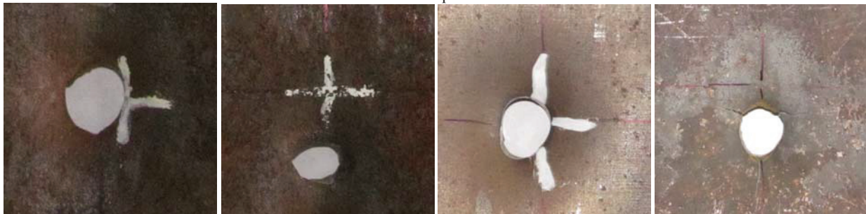
FIGURE 11. Results of the underwater interaction of SCM weighting about 150 g with steel obstacle of 8 mm in thickness at velocities about 500 m/s
