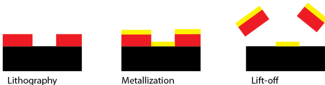
Figure 13. Lift-off process.
