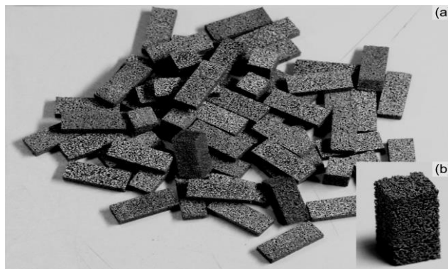
Fig. 1. Porous permeable TiNi-based alloy scaffolds (a) and single item (2.5x2.5x4 mm) (b) used in the study.
