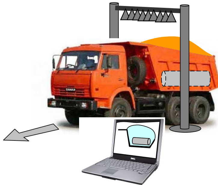
Figure 1. The hidden dielectric object in a metal body at the point of inspection.
