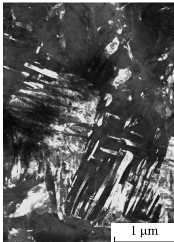
Fig. 3. TEM micrograph of the VT1-0 alloy surface after the action of 3 pulses.
