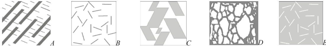
FIGURE 1. Test structures: St40-TiC (A, B, C), Aluminum foam (D), St40 with cracks (E)
