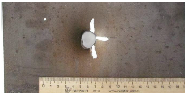
FIGURE 4. The barrier after interaction with the projectile
