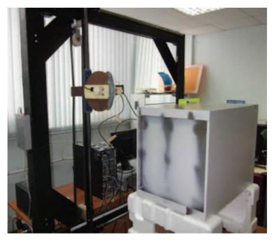
The system is basically a clocked array of UWB antennas, which are switched by electromechanical switching devices. When a truck moves through this system at low speed, it will be possible to sound the truck body in order to detect hidden objects under the load (soil, sand, etc.). A prototype of this system is shown in Fig. 8.4.
