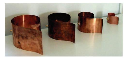
Fig. 8.9 UWB antennas of snail type
