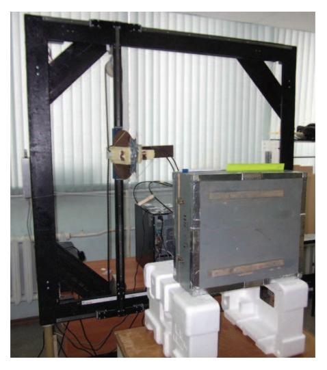
Fig. 8.17 UWB scanner and carrying box
