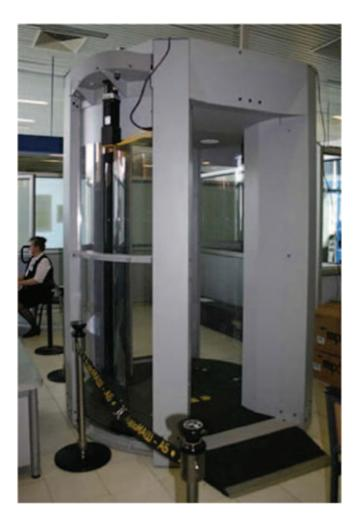
Fig. 8.1 The model of SafeScout 100 Scanner
