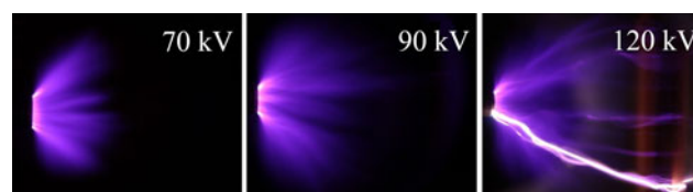
Fig. 10. Integral images of the discharge plasma glow at different voltage pulse amplitudes. The gap width is 6 cm. The exposure time is 1 s.
