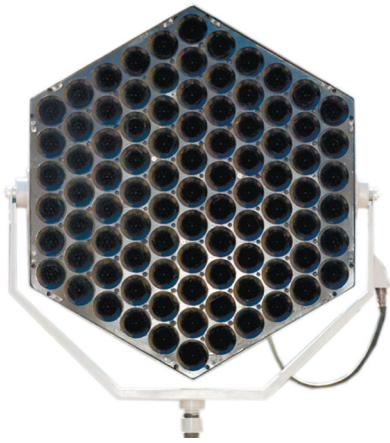
Fig. 1. Exterior view of the 91-element antenna array.
