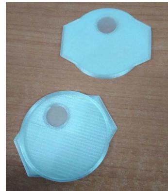
Fig. 1. Cuvette for measuring of the absorption of dry substances
