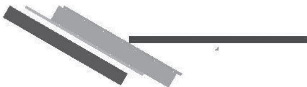
Figure 6. Interaction of projectile with the three-layer plate (middle layer – ceramics) at time t = 159 : initial system configuration “target – two plates + ceramics – projectile”.
