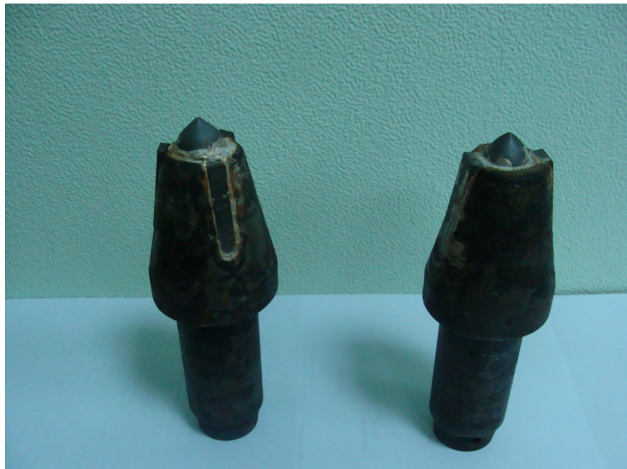
Figure 8. Coal machine cutters with heads reinforced by carbide blades
