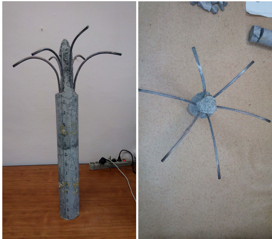
Fig. 12 Photographs of the reinforced concrete rod with a diameter of 104 mm, a length of 958 mm recovered after loading. Left—side view, right—top view
