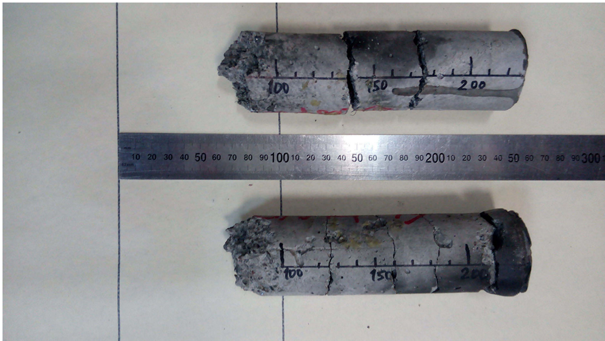
Fig. 7 Samples of concrete rods with diameter of 46 mm after the test on dynamic compression. The material of upper rod is concrete with steel fibers (the shot number C230f), for the lower sample it is concrete (C230)
