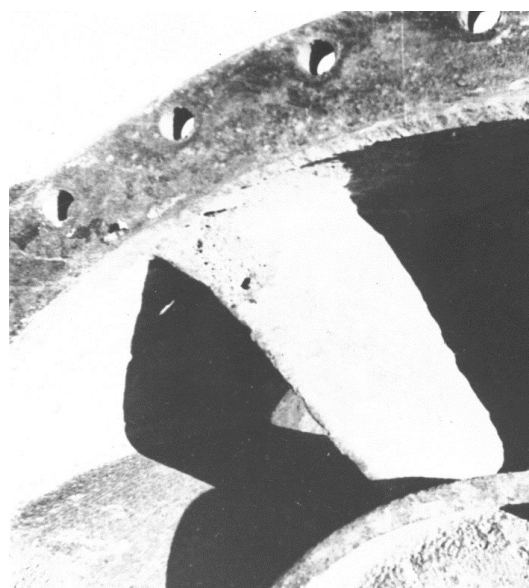
Fig. 6. Damage to the straightening apparatus of the OP10-185 pump of Kuyumazar PS after 6100 hours of operation
