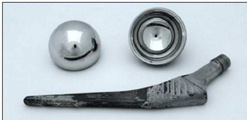
Figure 3. Elements of DePuy ASR TM XL total hip replacement: femoral head shown top left, acetabular cup shown top right and femoral stem shown in the bottom. Adapted from [39].
