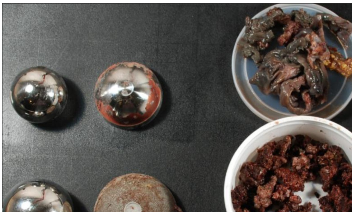
Figure 4. Explanted elements of DePuy's ASR hip implants and samples of fibrotic and necrotic tissue from the implantation site. [41]
