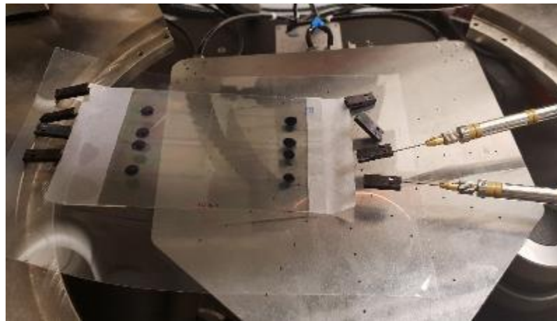
Figure 31. Probes connection to the final samples.
