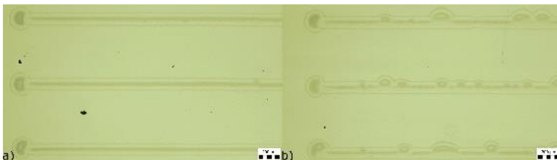
Figure 24. Two layers lines printed under the same conditions: a) uniform line; b) defects on the printed line.
