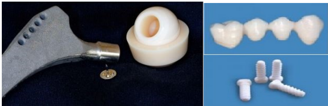
Figure 2. Dental implants and hip joint prosthesis made of alumina and zirconia based ceramics (Pina, et al., 2017).
