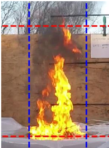
Figure 2 Illustration of automatically derived width (blue lines) and height (red lines) of the flame.
