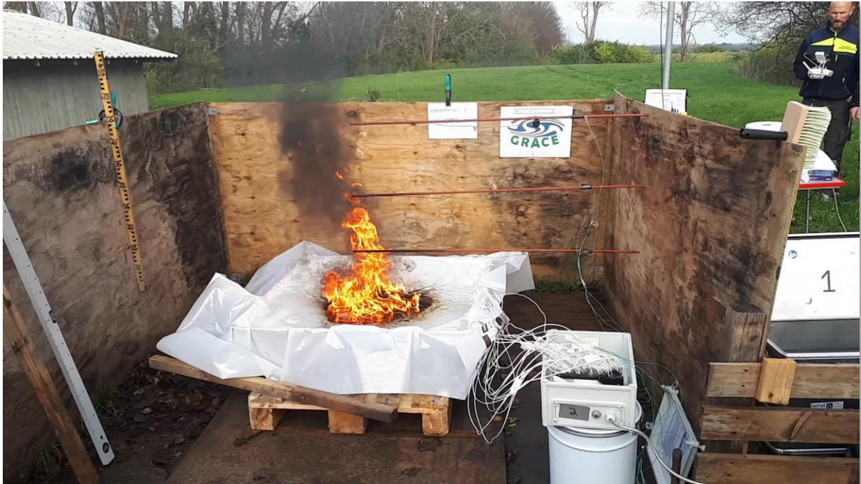
Figure 1 Overview of the burn experiment with ice pan and burning oil pool in the center.
