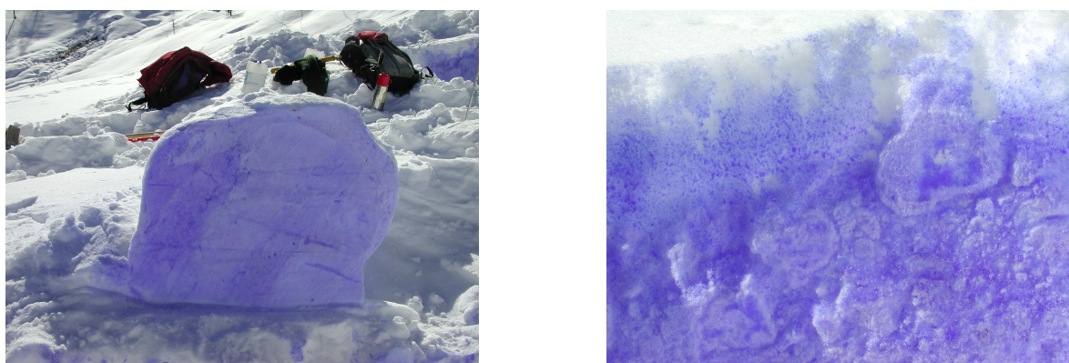
Figure 3. Cross-section and detail of a large snow clod in the run-out zone of the 10 February 2005 Salezertobel avalanche, Davos, Switzerland. The texture of the snow is made visible by spraying a mixture of ink and alcohol onto the smoothed surface, warming it carefully with a camping cooker and waiting for the ink to diffuse into the snow by capillary suction. Note the layered core (oblique stripes (left) and the small snow clods sintered onto it (right).
