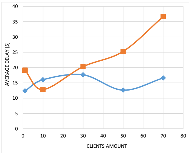
Apache Server latency for handling requests for medium size resource – binary file, size 28 MB (■ – 30 threads, ◆ – 150 threads)
