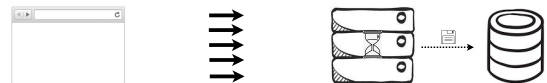
Figure 4: Running multiple concurrent user traces against the web application. An active query delay is active to force the exploitative interleaving needed to validate the GRC. The occurring sql log data is collected
