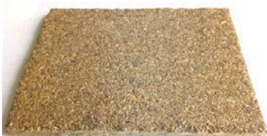
Figure 45: Photos of the samples of the adhesive (alkaline aluminosilicate binder) bonded wood-based materials: particle boards and (left) plywood after testing for internal bond (right)
