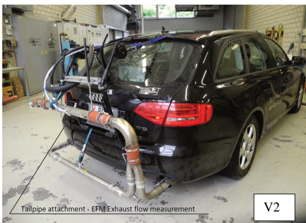
Fig. 3. Tested vehicles (FFV) equipped with PEMS
