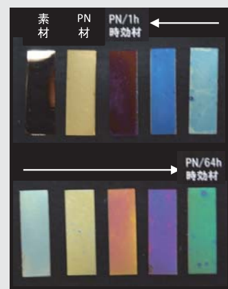
耐摩耗性と意匠性を付与した高強度銅合金 Colored copper alloys with high-strength and toughness
