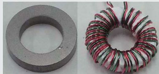
コアの外観写真。(左) 成形体、(右) 製品体 Outer appearances of (Left) consolidated core and (Right) core product.
