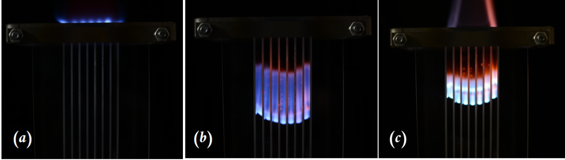
Fig. 4. Photographs of the multi-channel burner in configuration I obtained for Q = 405 \text{ cm}^3/\text{s} ( U = 32.1 \text{ cm/s} ) and \phi = 0.7 (a), \phi = 0.8 (b), \phi = 1.2 (c).
