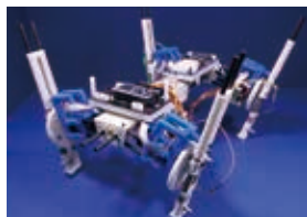
Quadruped robot that exhibits gait transition
