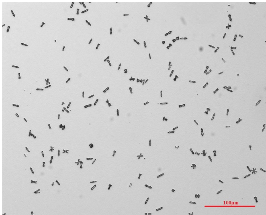
Figure 3.44: 0.2 mM of Zinc-cystine microparticles in sterilized water in the incubator (37 °C). The picture was taken 3 hours after microparticles were added into the plate. 10x magnification.
