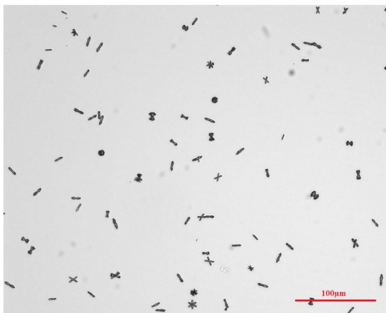
Figure 3.46: 0.2 mM of Zinc-cystine microparticles in the astrocyte cell culture media in the incubator (37 °C). The picture was taken 3 hours after microparticles were added into the plate. 10x magnification.
